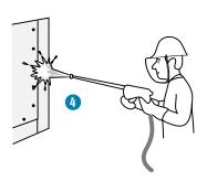
4. Rinse throughly with a high-pressure water jet. Treat the waste water before discharge.
