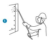
1. Apply the Cleaner with a brush or by spraying or dipping.
